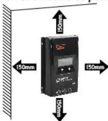
Figure2-1 Mounting
